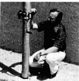
Hinged Base Plate - Concrete Pad, Heavy Duty Winch
